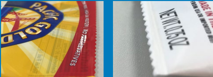
Thermally welded seals (left) are wider than ultrasonics seals (right) due to the risk of contamination in the sealing area.
