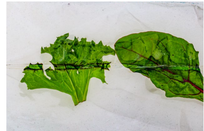
Contamination during thermal sealing processes affects the tightness of the packaging.
