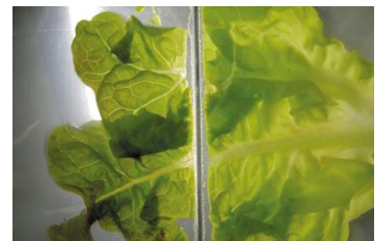
Ultrasonics displace product residues from the sealing area.
